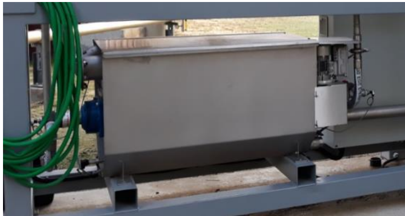
Figure 7. Heater exchanger integrated into the skid
