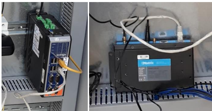
Figure 13. Embedded pc (left) and 3G router (right)
