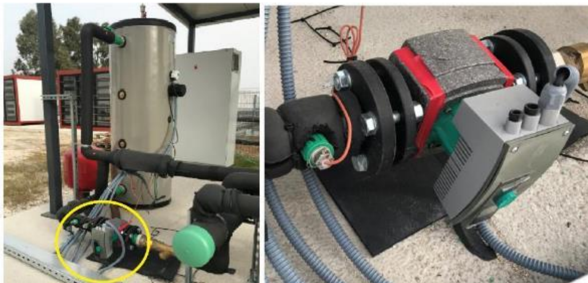
Figure 24. The pump of emulation tank (P2)
