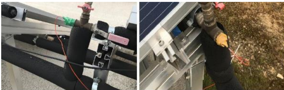
Figure 31. Temperature sensor distributed in the solar field
