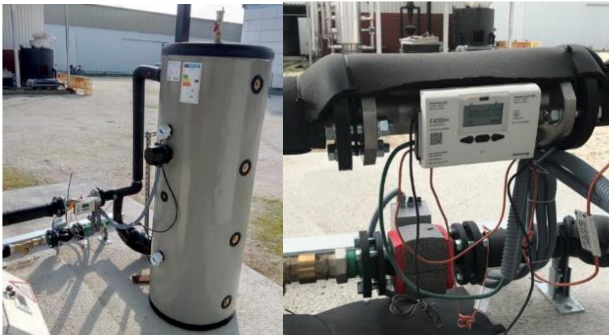
Figure 18. Emulator tank and its pumps and flow rate meter
