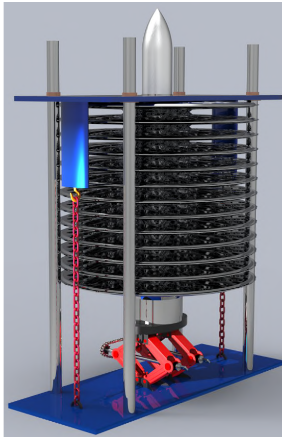
Picture 47: The mounting rig acting on a 10-disk rotor.
