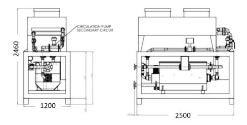
Figure 5. Heat recovery system skid dimensions.
