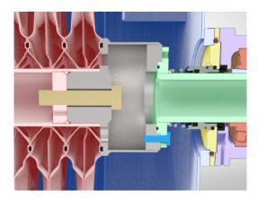
Picture 46: Rotor end-cap section.
