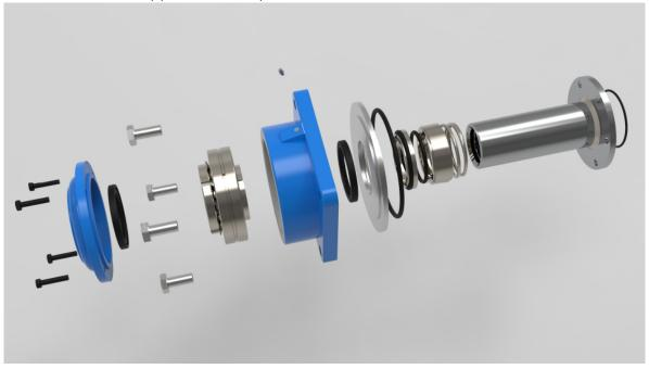
Picture 39: The non-drive-side support assembly.
