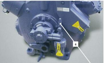
Figure 6: Pre-lubrication valve (6)
