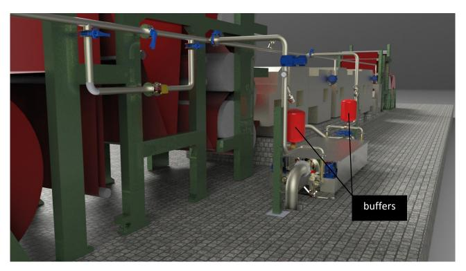
Picture 13: Exchanger with buffers
