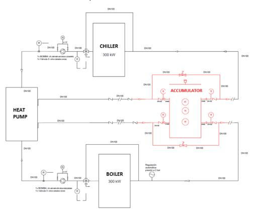
Figure 21. Installation scheme of HP-LowUP concept in Guipuzkoa.
