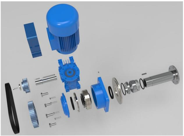
Picture 37: The drive-side support assembly
