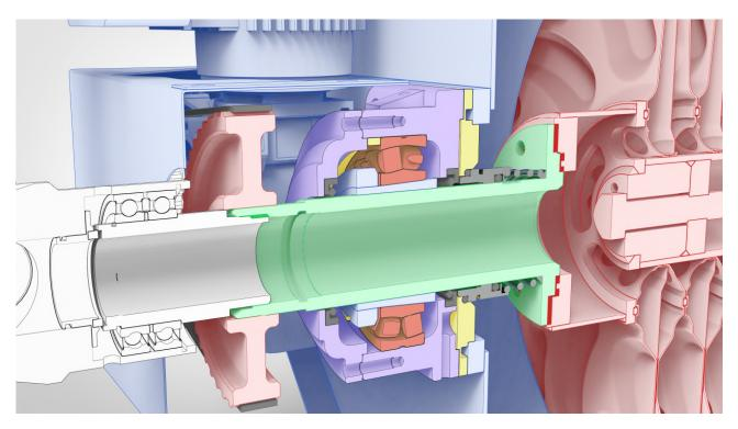
Picture 38: Moto-reducer side support section
