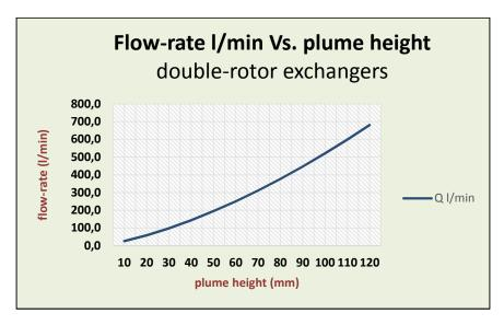
Picture 11: Flow-rate measure (double rotor)
