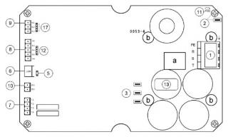
Picture 44: Inverter board connections
