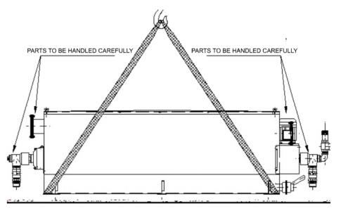
Picture 15: Handling of the unpacked unit.
