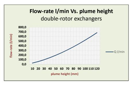
Picture 11: Flow-rate measure (double rotor)
