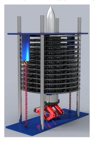
Picture 47: The mounting rig acting on a 10-disk rotor.
