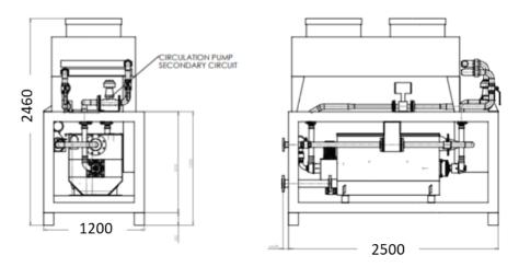
Figure 15. Heat recovery system skid dimensions.
