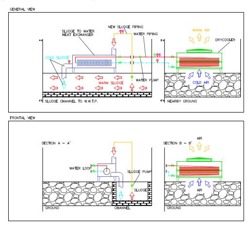
Figure 13. Setubal Demo Site P&ID conceptual diagram.
