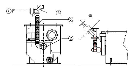
Picture 23: Flex pipe correct installation.
