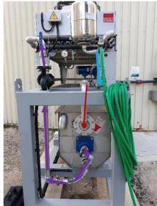
Figure 11. Liquid flow scheme of heat exchanger.
