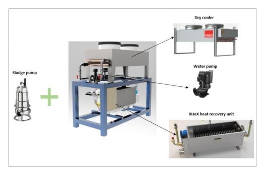
Figure 14. Integration unit and systems of Setubal demo site.
