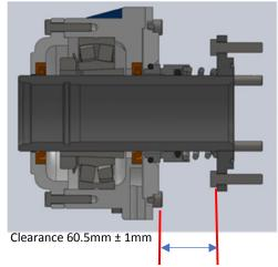
Picture 26: Seal pre-charge clearance
