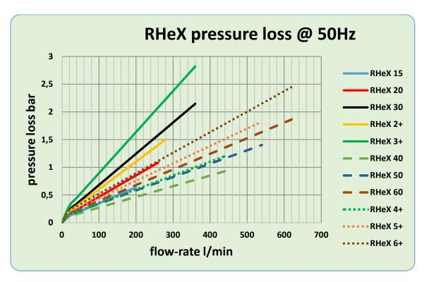
Picture 12: Secondary circuit pressure loss (all models)
