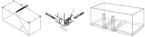
Figure 4: Bottom lift sling method & Fork lift method
