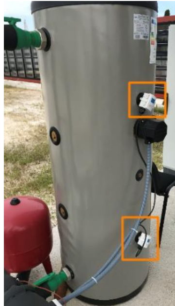
Figure 71. Temperature sensor inside Wasenco emulator.
