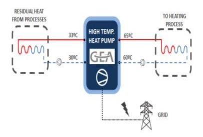
Figure 34. LowUP system for wastewater treatment plant
