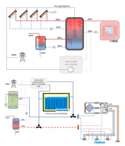
Figure 29. LowUP technologies for demo 1. Heat LowUP (Top) and Cool LowUP (Bottom)
