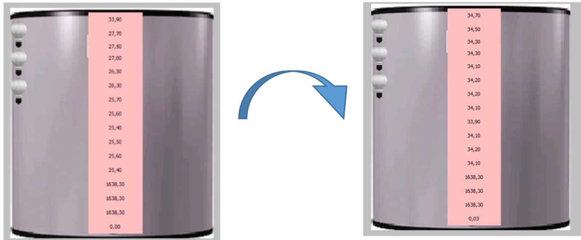
Figure 77. Temperature sensors distributed in Stratified tank
