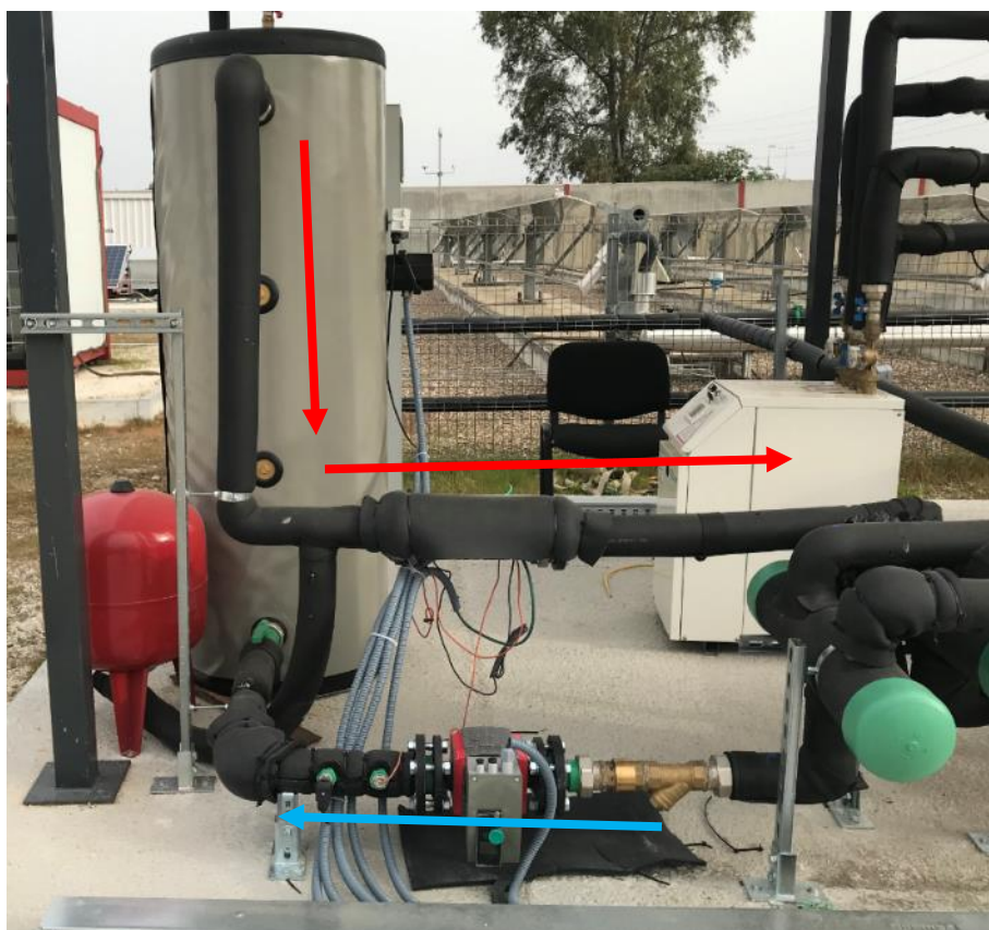
Figure 70. Schema of the inlet (blue) and outlet (red water) from emulator to tank
